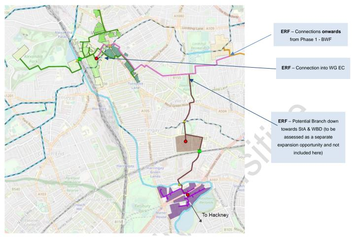
Figure 2.33 – ERF Option (2) – Interconnector Pipework Potential Routes
